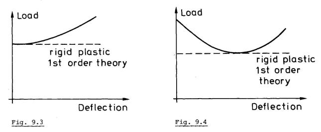
The maximum load found for the clamped slab will not be reached in practice because of the elastic deformations neglected.
