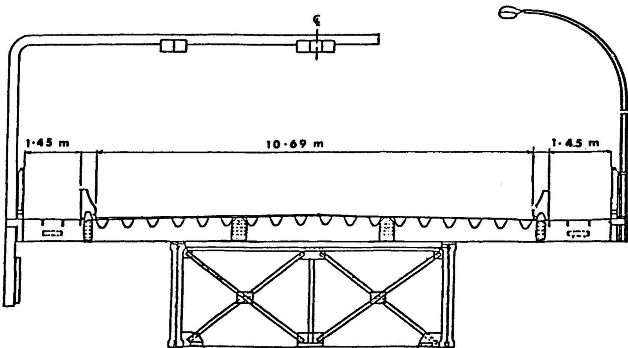
Fig. 4 Cross Section of Renovated North Viaduct
