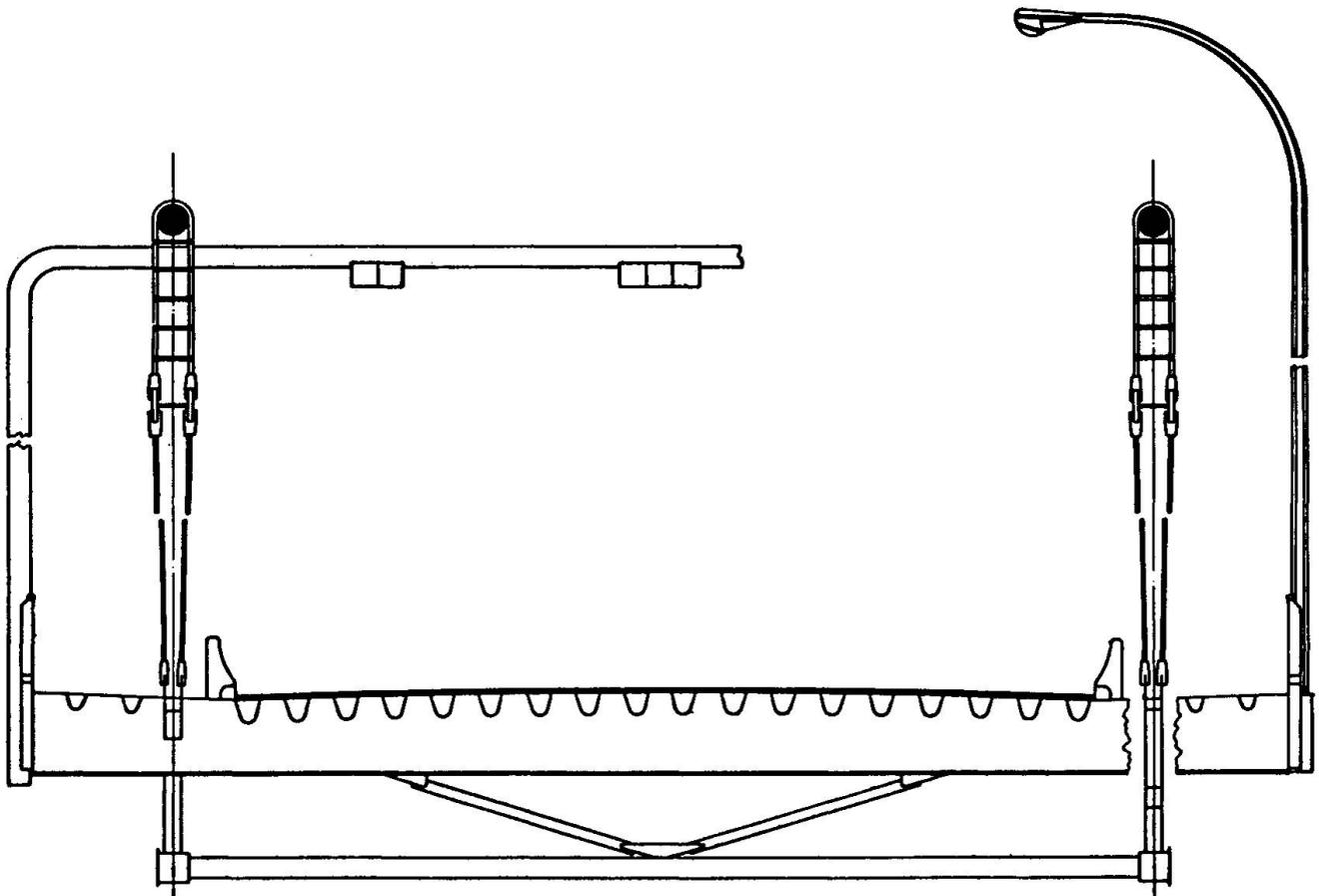
Fig. 7 Suspension Bridge New Stiffening Truss Section
