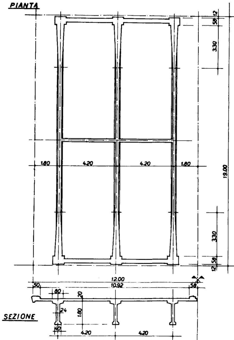
Fig. 1 - Geometry of the standard bay.
