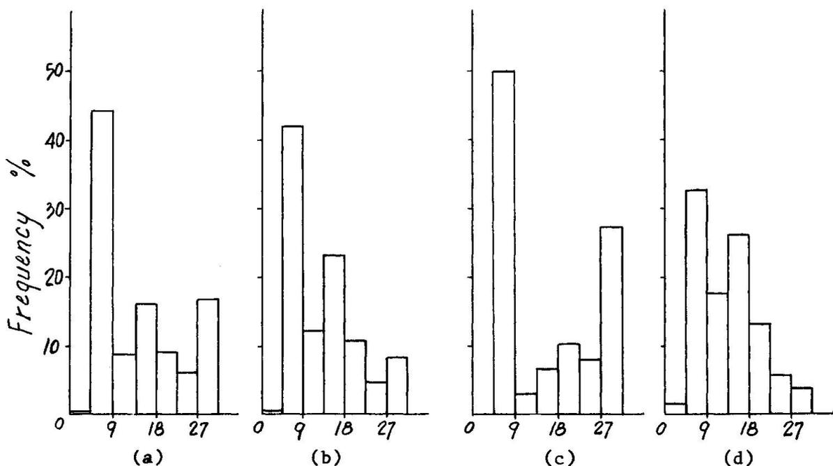
Fig. 1 Axle Load Histograms (Metric Tonnes)
