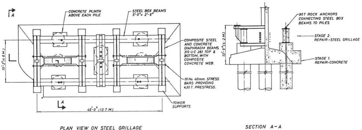
Fig. 6 Pile Cap 20. Temporary steel cap
