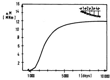
Fig. 10 Changes of the bending moment in the middle of the third span of the bridge
