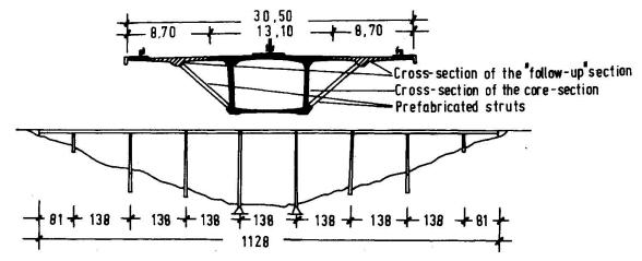
Fig. 7 Cross-section and side view of the Kocher Valley Bridge
