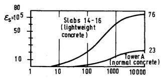
Fig. 4 Shrinkage of normal and lightweight concrete
