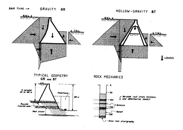
Fig. 3.1 - Investigation on dam-foundation complex
