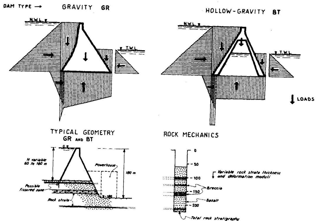
Fig. 3.1 - Investigation on dam-foundation complex
