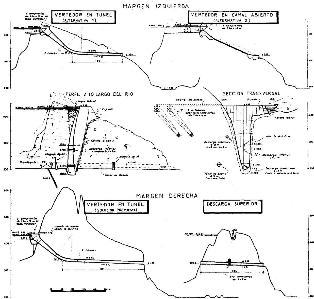
Fig. 3.3 - Study of dam-spillway alternatives. Sections
