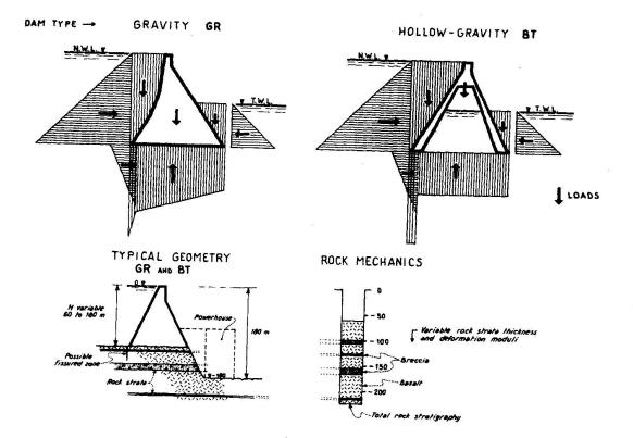
Fig. 3.1 - Investigation on dam-foundation complex
