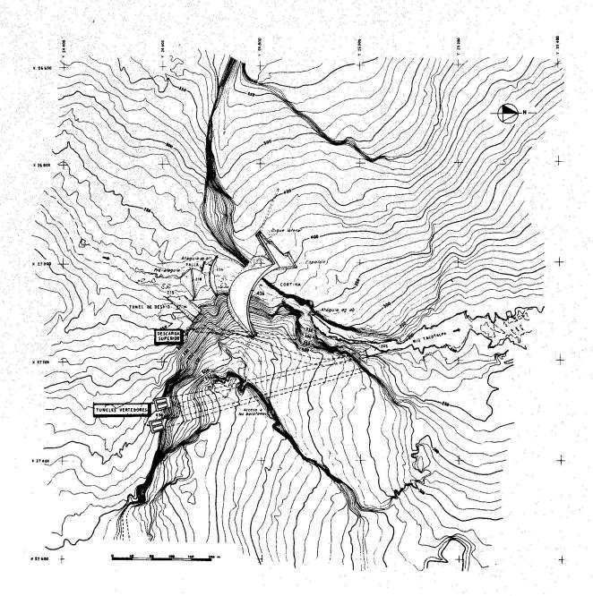
Fig. 3.2 - Study of dam-spillway alternatives. Layout
