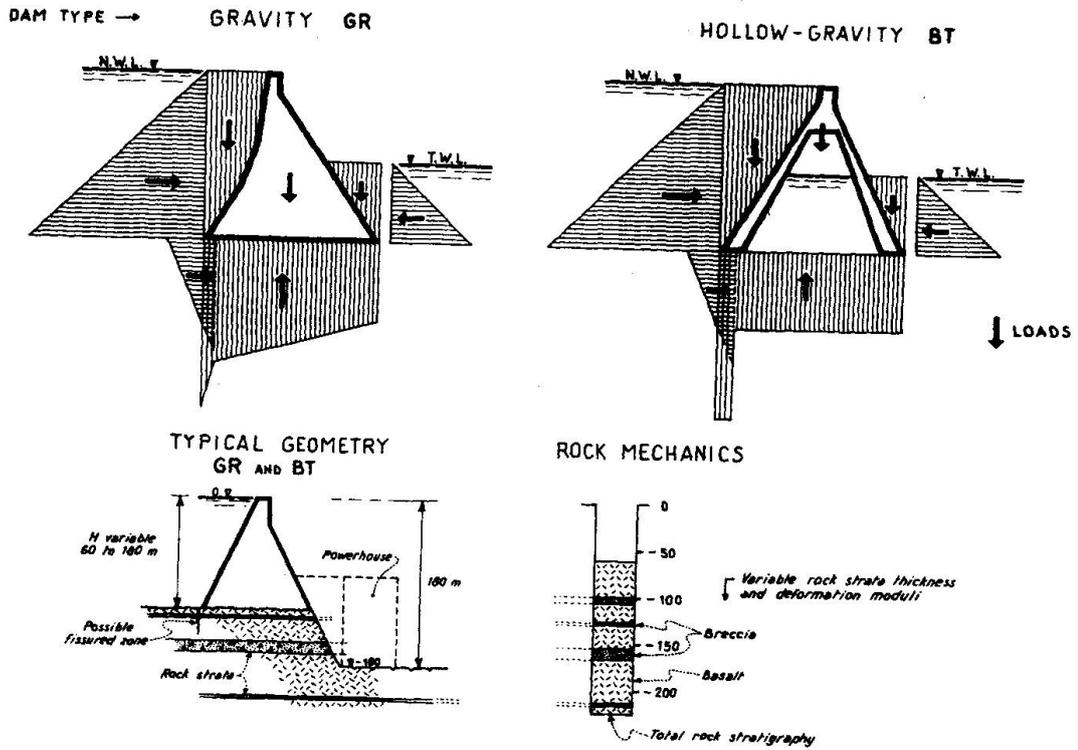
Fig. 3.1 - Investigation on dam-foundation complex
