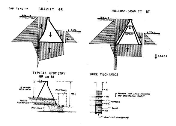
Fig. 3.1 - Investigation on dam-foundation complex
