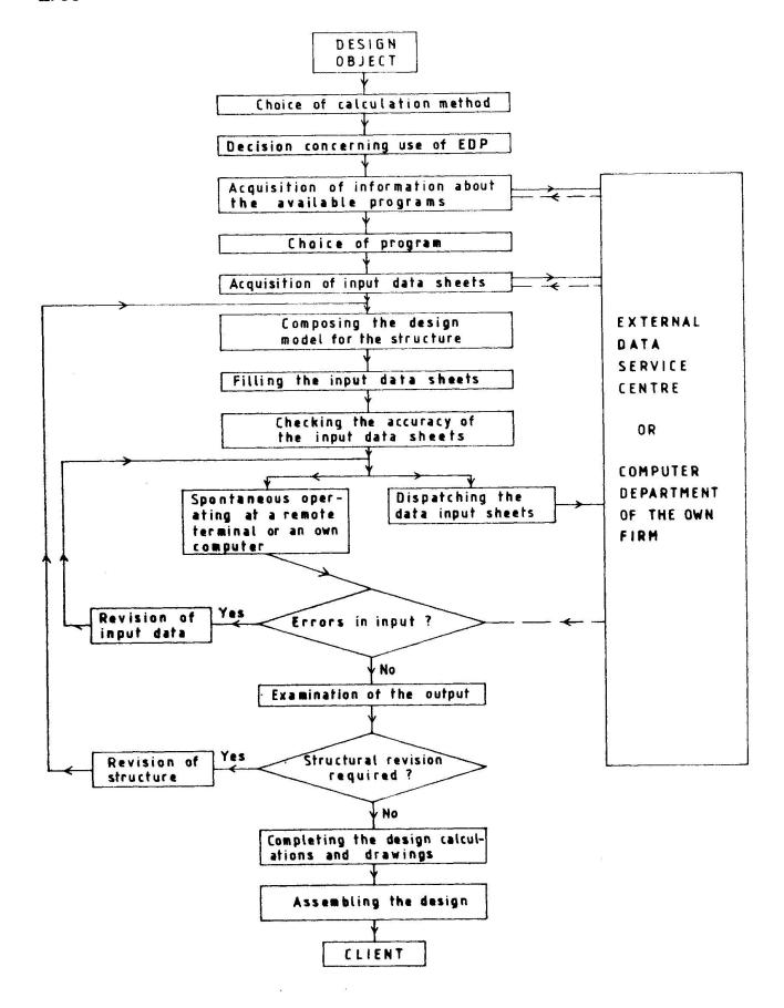
Fig. 1 Computation procedure in structural design with or without personally operating the computer.
