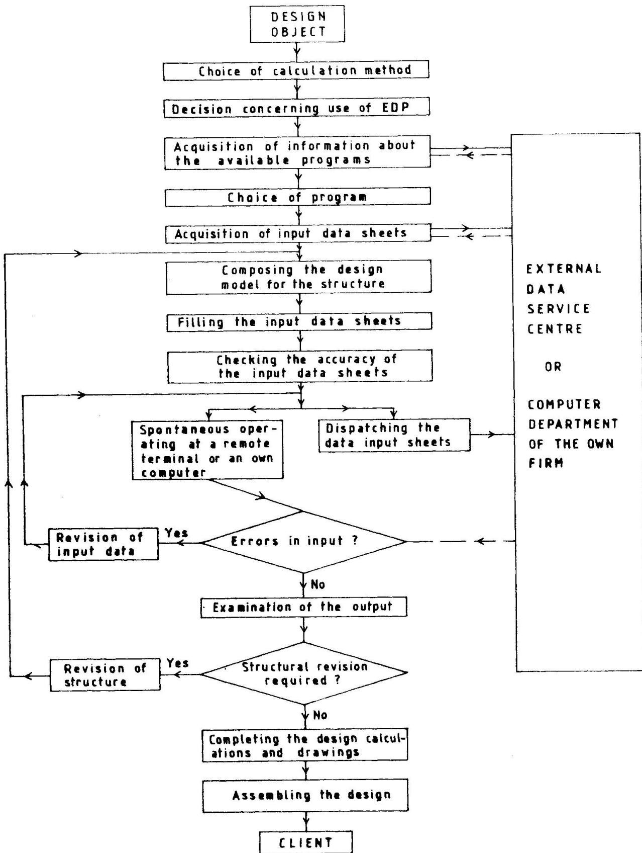
Fig. 1 Computation procedure in structural design with or without personally operating the computer.
