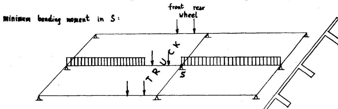
Fig.1: T-shaped beam: taking into account corresponding single loads by evaluating the lines of influence
