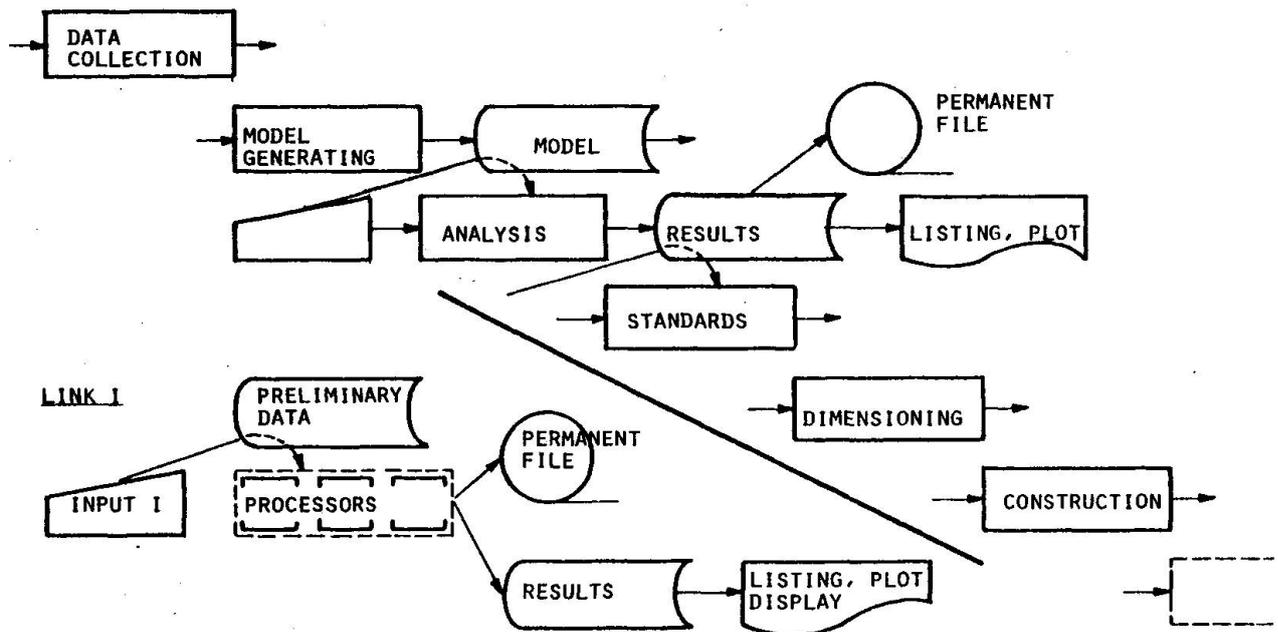
**Fig. 1** Scheme of the Design Process
