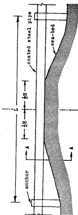
FIG. 1a Pipe-seabed configuration under consideration.
