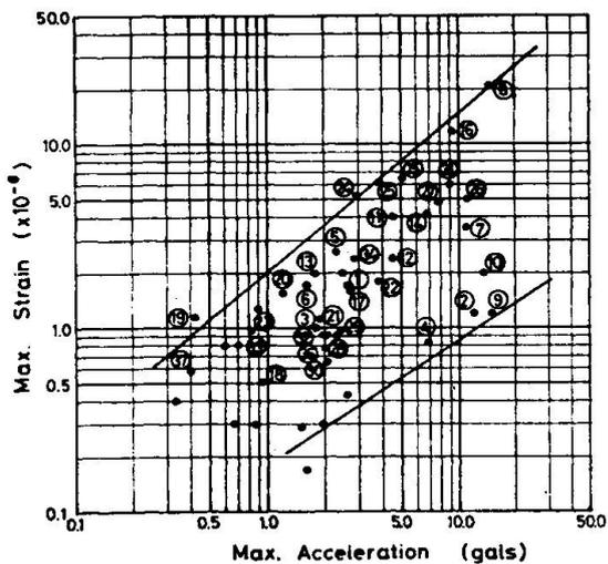
Fig.3 Relation between max.acceleration and max.axial strain at Haneda Tunnel (J.N.R.)
