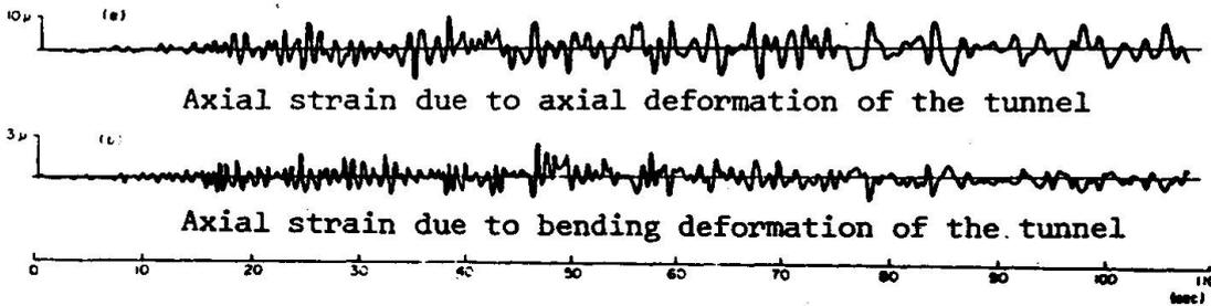
Fig. 7 Strain waves generated by axial deformation and bending deformation of tunnel (Haneda Tunnel) during earthquake (December 4, 1972) and their power spectra
