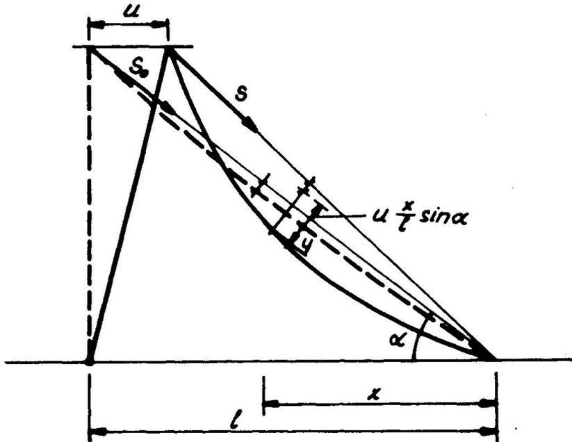
**Fig. 1** Displacement of one guy of the support
