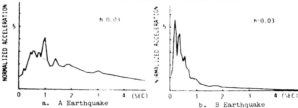
Fig. 10 Acceleration Spectra of Observed Earthquake (Transverse)
