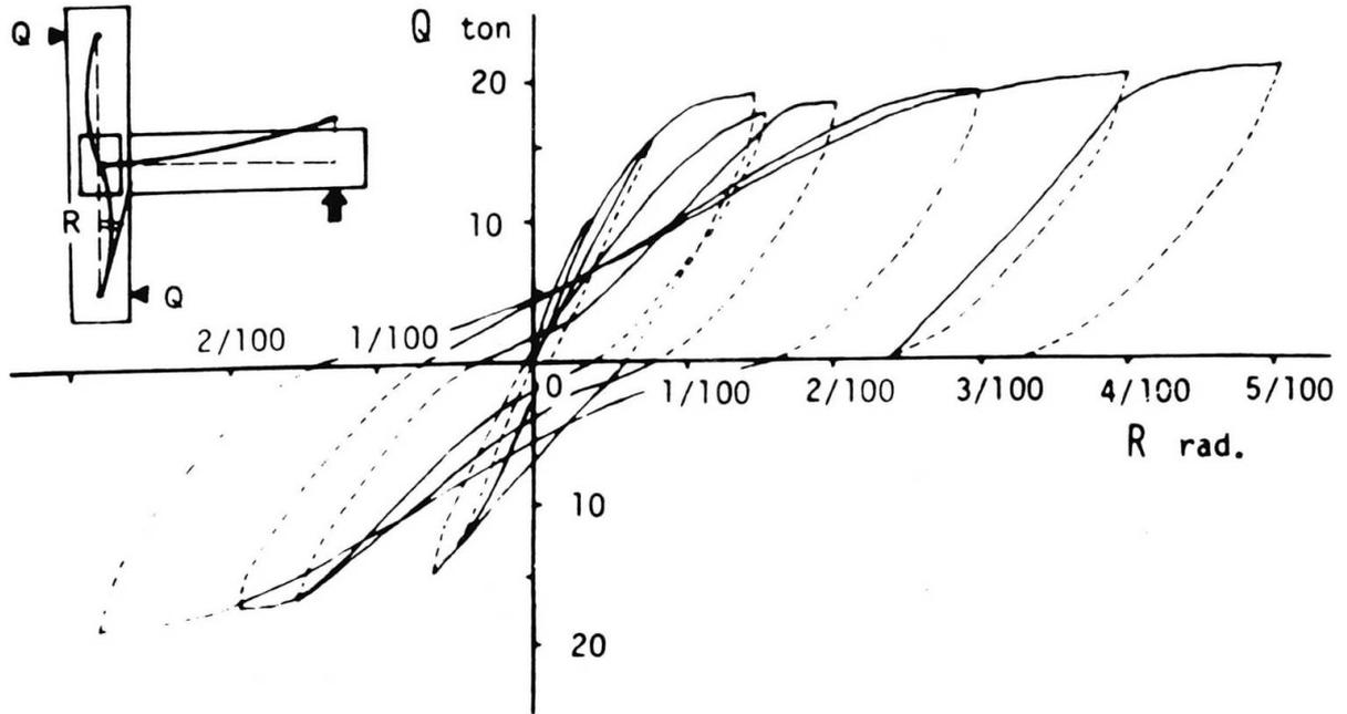
Fig. 2 Load-Deflection Curve of Exterior Framing including U Anchor Method
