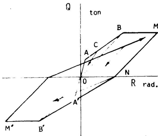
Fig. 6 Idealized Hysteresis Loop of Shear Stiffness
