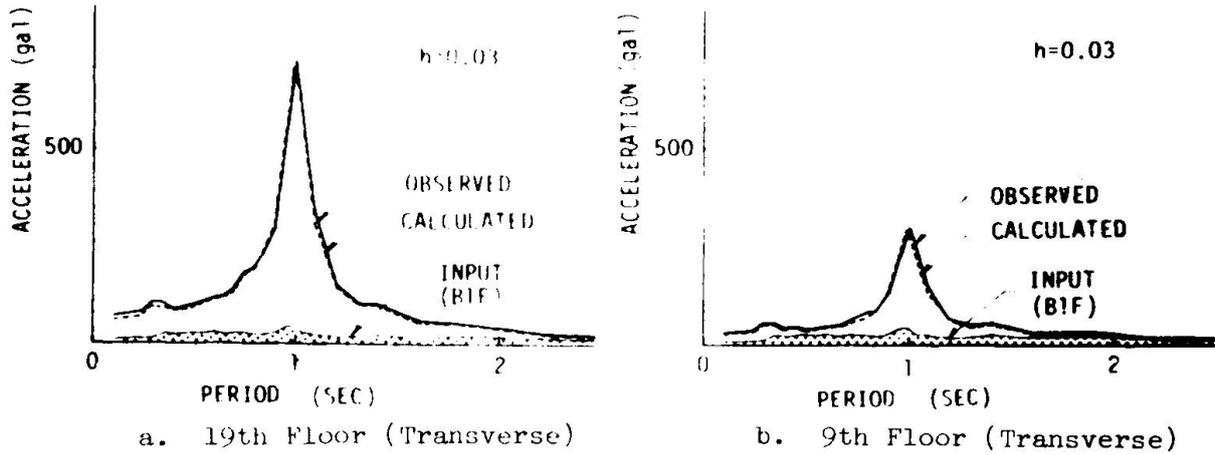
Fig. 12 Comparison of Acceleration Spectra (A)
