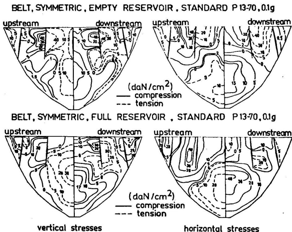
Fig. 8 Vidraru dam, the structure with partially grouted joints and crest belt: Isolines of horizontal and vertical normal seismic stresses.
