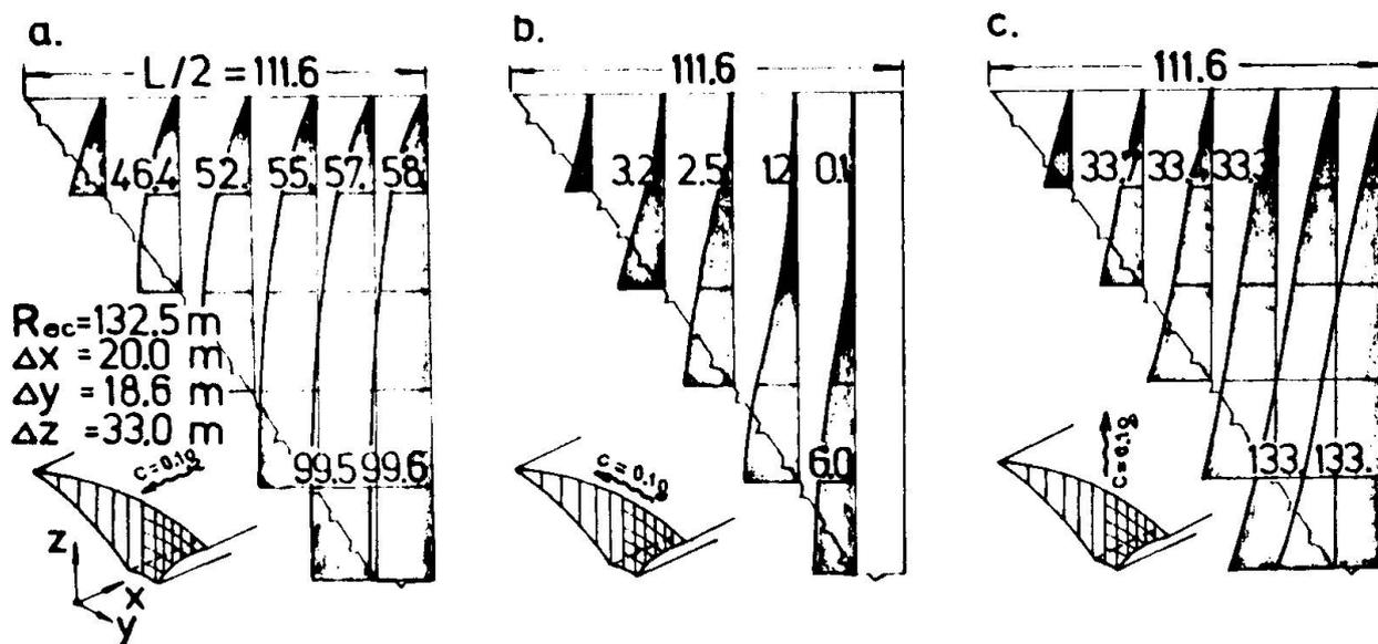
Fig. 3 Variation of velocity potential function  $\Psi$  on the Vidraru dam halfstructure subjected to earthquakes on the directions: a-horizontal, along the valley, b-horizontal, transverse the valley, c-vertical.
