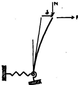
Figure 6: Structural model to calculate the force-deflection-relationship
