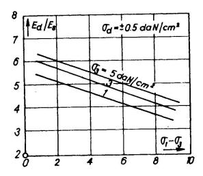
Fig. 1 The correlation between E<sub>d</sub>/E<sub>s</sub> ratio and the principal stresses in the dam body (after Hayashi, Fuziwara and Komeda).
