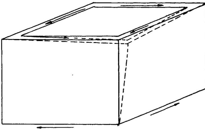
Figure-2 Corner Behaviour of Masonry Buildings.
