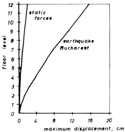
Fig.5 Envelopes of maximum elastic floor displacements
