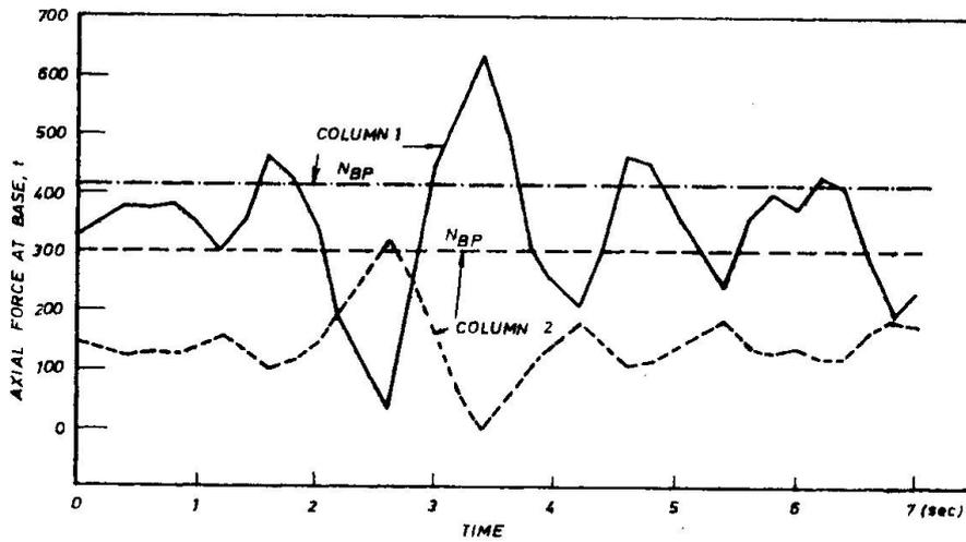
Fig.11 Time history of axial forces at base of D<sub>2-3</sub>
