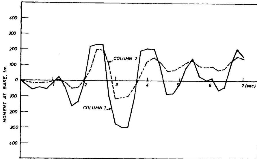
Fig.10 Time history of bending moment at base of D<sub>2-3</sub>
