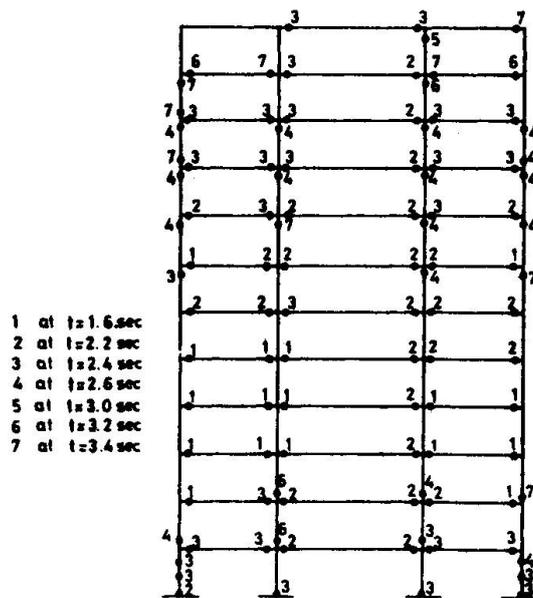
Fig.12 Sequence and location of plastic hinges, D<sub>2-3</sub>
