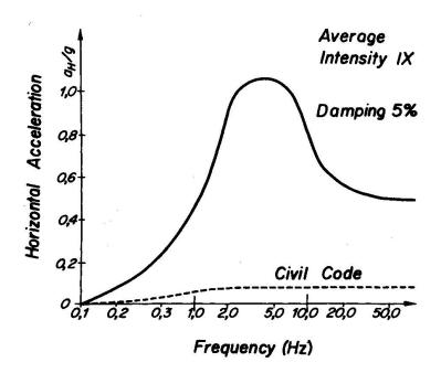
Figure 21: Horizontal ground acceleration for earthquakes of intensity IX (MSK) (U.S. Atomic Energy Commission, WASH 1255). The dashed line gives the disign ground acceleration according to the conventional aseimic building code.
