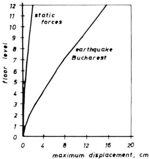
Fig.5 Envelopes of maximum elastic floor displacements
