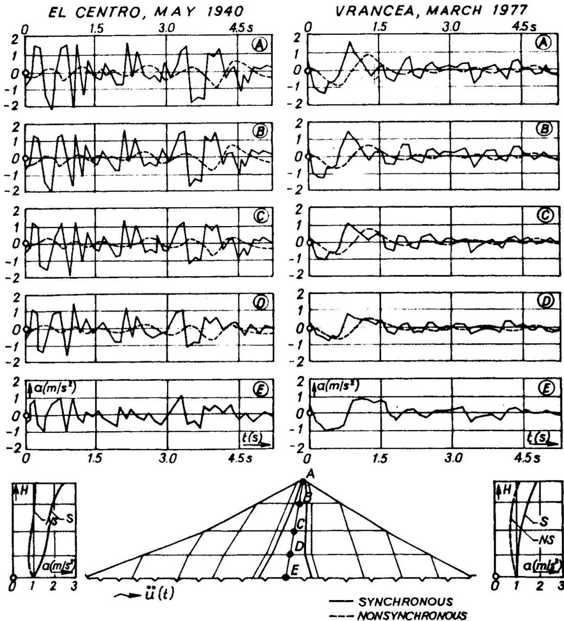
Fig. 6 The influence of the nonsynchronous character of the excitation on the earthquake response of Lotru dam.
