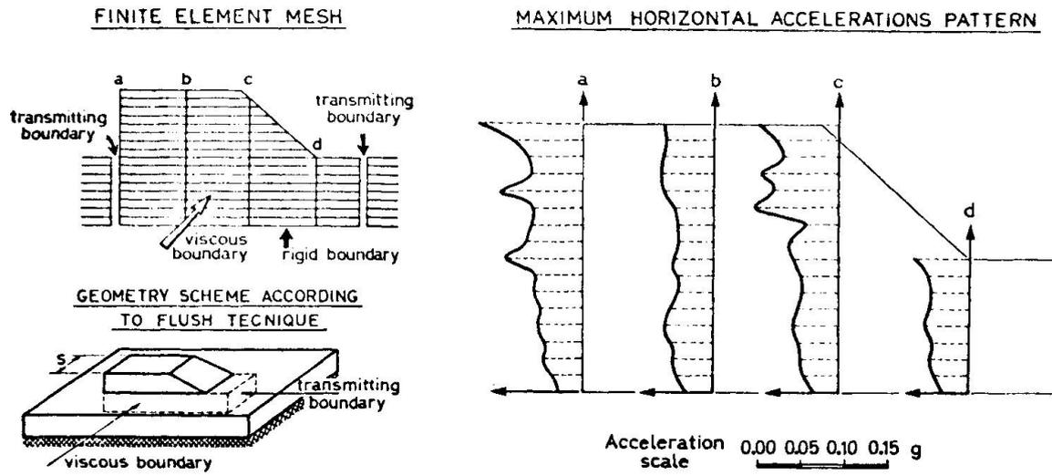
Fig.10 - Hilly site. Geometric effect on accelerations
