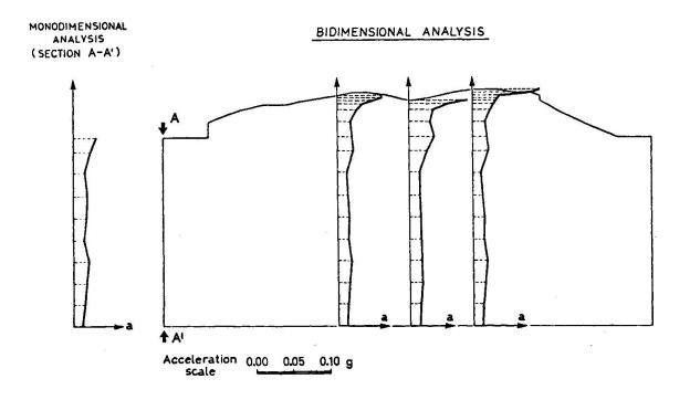
Fig. 2 - Buia hill. Comparison of accelerations obtained with monodimensional analysis
