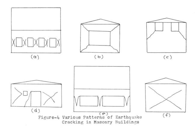
of the cracks will be influenced by the height to width ratio of the wall and location and size of the window and door openings. Figure-4.
