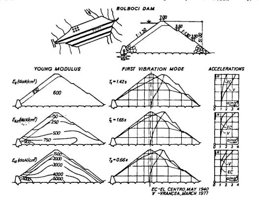
Fig. 4 Earthquake response of the Bolboci dam.
