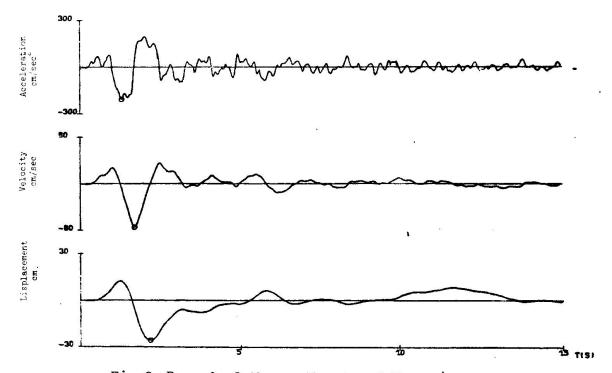
Fig. 2 Record of the earthquake of March 4,1977 - INCERC
