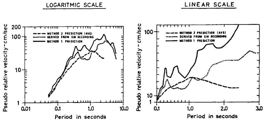
Fig.7 - Calculated relative site transfer function and comparison of spectral prediction methods - Hays et al. results [11]
