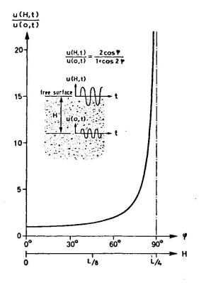
Fig. 8 - Frequency transfer function
