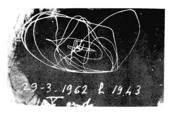
Fig. 5: Seismoscope record of a 4.3 magnitude earthquake.
