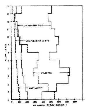
Fig.7 Envelopes of maximum storey shears
