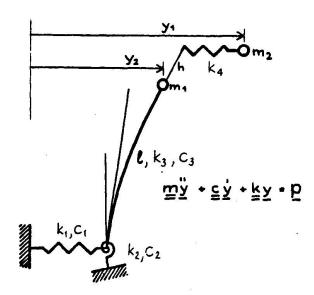
Figure 8: Structural system of Gemona watertower for elastic response analysis;  $m_1$  is the sum of the weight of the structure and Housner's added mass for impulsive pressure;  $m_2$  and  $k_2$  account for the added mass-spring-system resulting from the convective pressure in the composite combiner.
