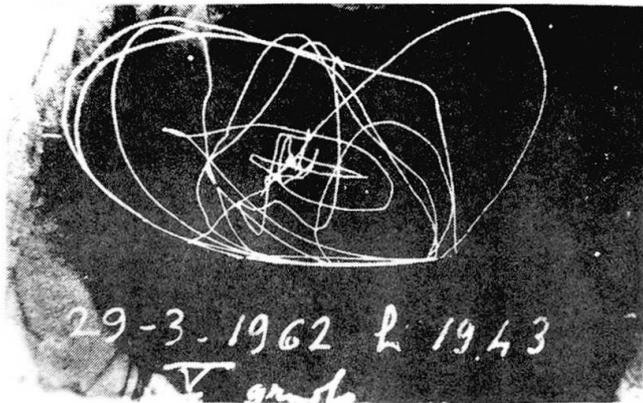
Fig. 5: Seismoscope record of a 4.3 magnitude earthquake.
