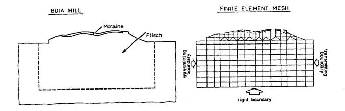
FIG. 1 - Buia hill. Geometry and finite element mesh
