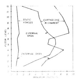
Fig.6 Envelopes of maximum beam ductilities, D<sub>2-3</sub>
