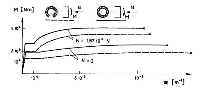
Figure 5: Momentum-curvature-relationship for the reinforced concrete column. The normal force  $N = 1.97 \cdot 10^6 \ N$  is the result of water and structure weight.
