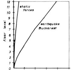
Fig.5 Envelopes of maximum elastic floor displacements
