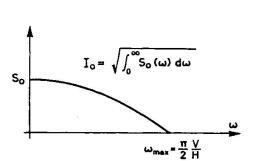
Fig. 9 - Assumption for power spectral density of seismic acceleration at some depth
