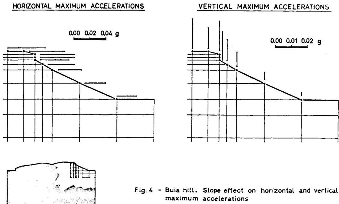
Fig.4 - Buia hill. Slope effect on horizontal and vertical maximum accelerations
