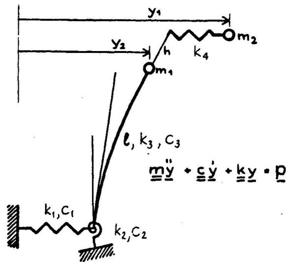
Figure 8: Structural system of Gemona watertower for elastic response analysis;  $m_1$  is the sum of the weight of the structure and Housner's added mass for impulsive pressure;  $m_2$  and  $k_2$  account for the added mass-spring-system resulting from the convective pressure in the composite combiner.
