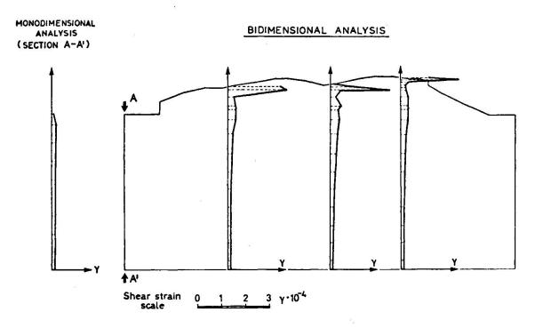
Fig. 3 - Buia hill. Comparison of shear strains obtained with monodimensional and bidimensional analysis
