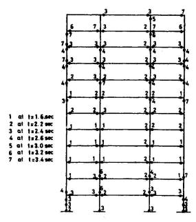
Fig.12 Sequence and location of plastic hinges,  $D_{2-3}$
