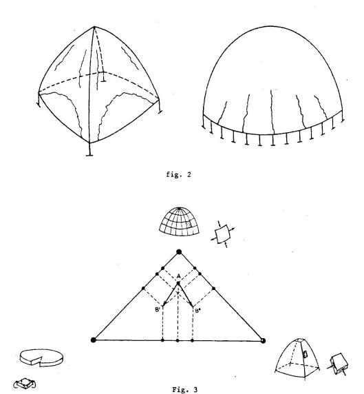
For any modification of the physical state of the vault (e.g. cracks or partial collapses) there will be a variation of the tri-partition: the representative point will pass in B" (increase of the plate effect produced by settling of the bearing structures or by arched cracks on the base of the vault); or in B' (increase of the slab effect revealed first by cracks in accordance with the meridians).
