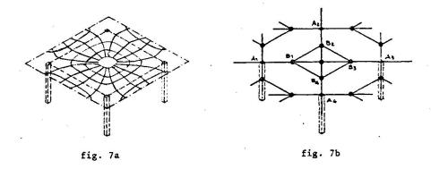
generical field of the continuous slab and part of the adjacent fields. Then in fig. 7d the lines of fracture of a single field with some adjacent elements have been constructed.
