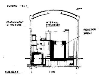
Fig. 2 - Reactor Building Plan and Elevation
