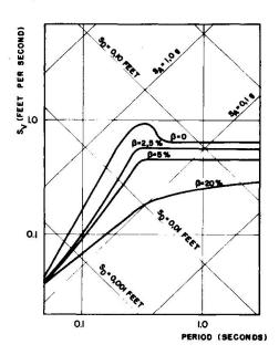
Fig.3 - Design Basis Earthquake Spectrum
