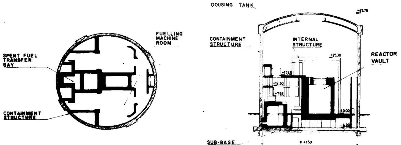
Fig. 2 - Reactor Building Plan and Elevation
