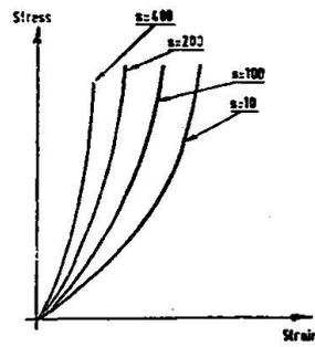
Fig. 2. Typical stress-strain compression curves of isolators.
