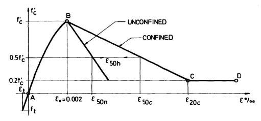
Fig. 1. Stress-strain curve for confined concrete
