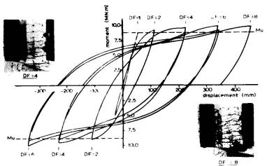
FIG 1: Moment-Displacement Loops for Unit 4, after Priestley et al [1]
