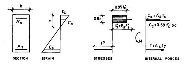
Fig. 3. Scheme for computation of a monotonously loaded reinforced concrete section
