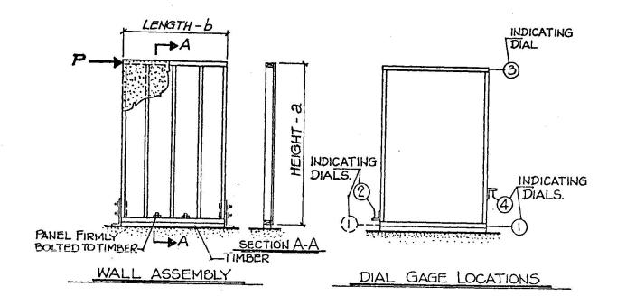
Figure 1. Racking Load Assembly ASTM E 564 - 76.
