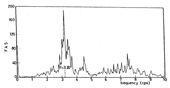
Fig. 4 Fourier amplitude spectra on the ground floor
