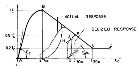
Fig. 4. Stress-strain behavior of concrete with cyclic loading
