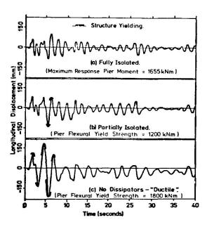
FIG 9: Longitudinal Response of Bridge for Three Structural Alternatives (El Centro 1940 N-S)
