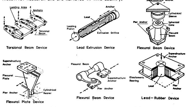
FIG 6: Schematic Drawings of Mechanical Energy Dissipating Devices
