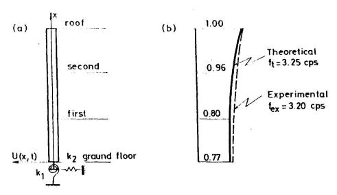
Fig. 6 (a) Cantilever beam model with interactive parameters
