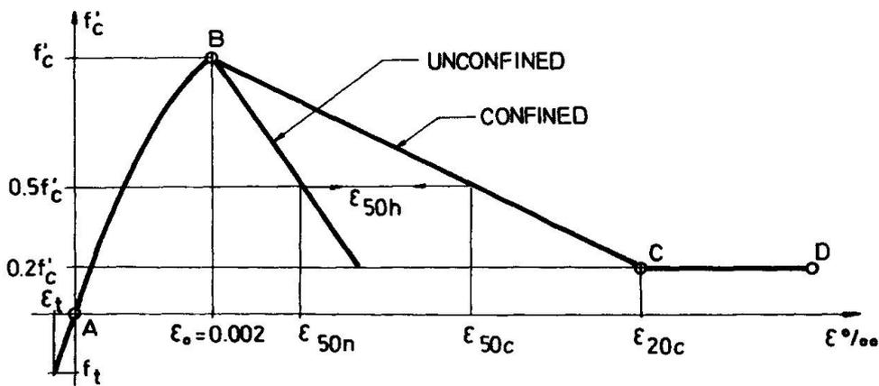
Fig. 1. Stress-strain curve for confined concrete
