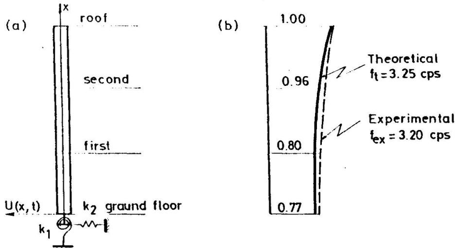
Fig. 6 (a) Cantilever beam model with interactive parameters
