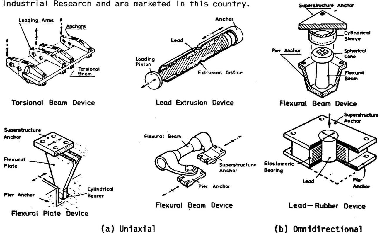
FIG 6: Schematic Drawings of Mechanical Energy Dissipating Devices
