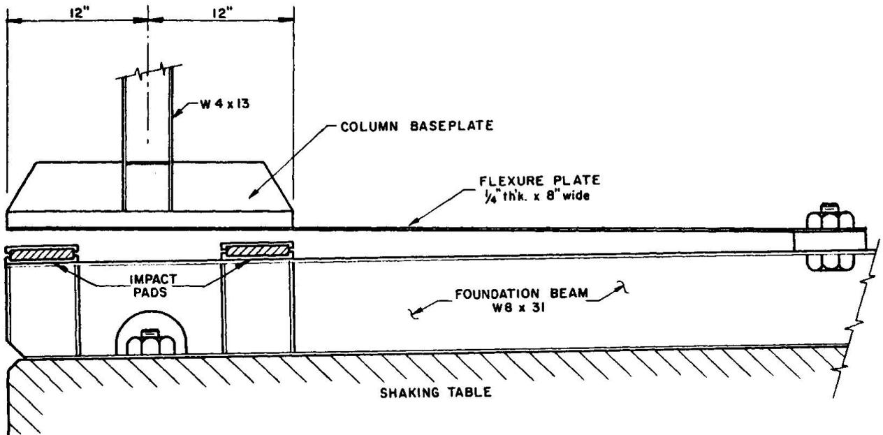
Fig. 3 Uplifting Column Base Detail
