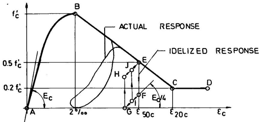
Fig.4. Stress-strain behavior of concrete with cyclic loading
