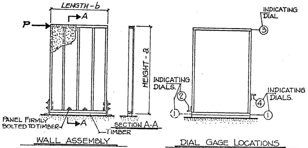
Figure 1. Racking Load Assembly ASTM E 564 - 76.
