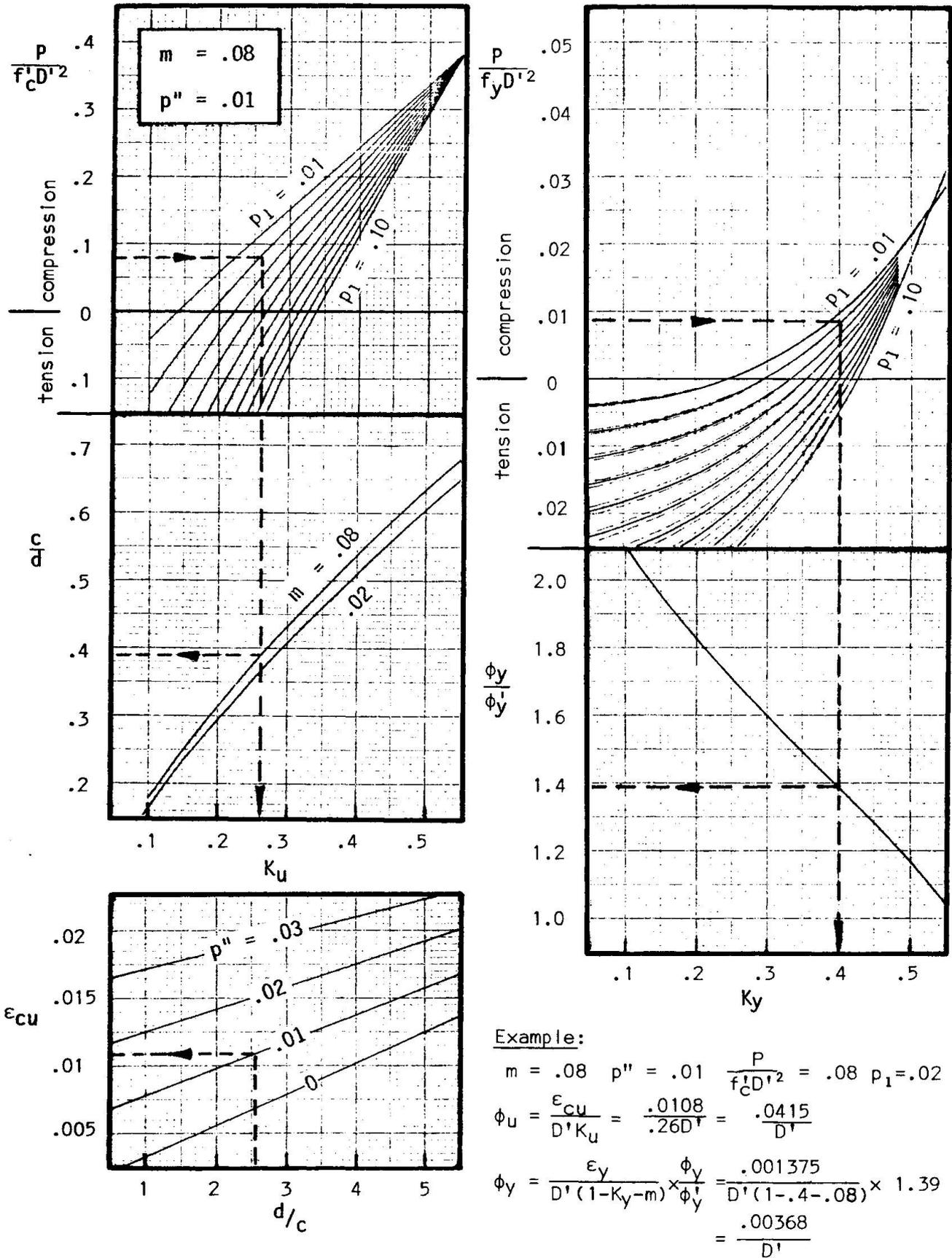
FIG 5: Example Charts for Calculation of Curvature Ductility.
