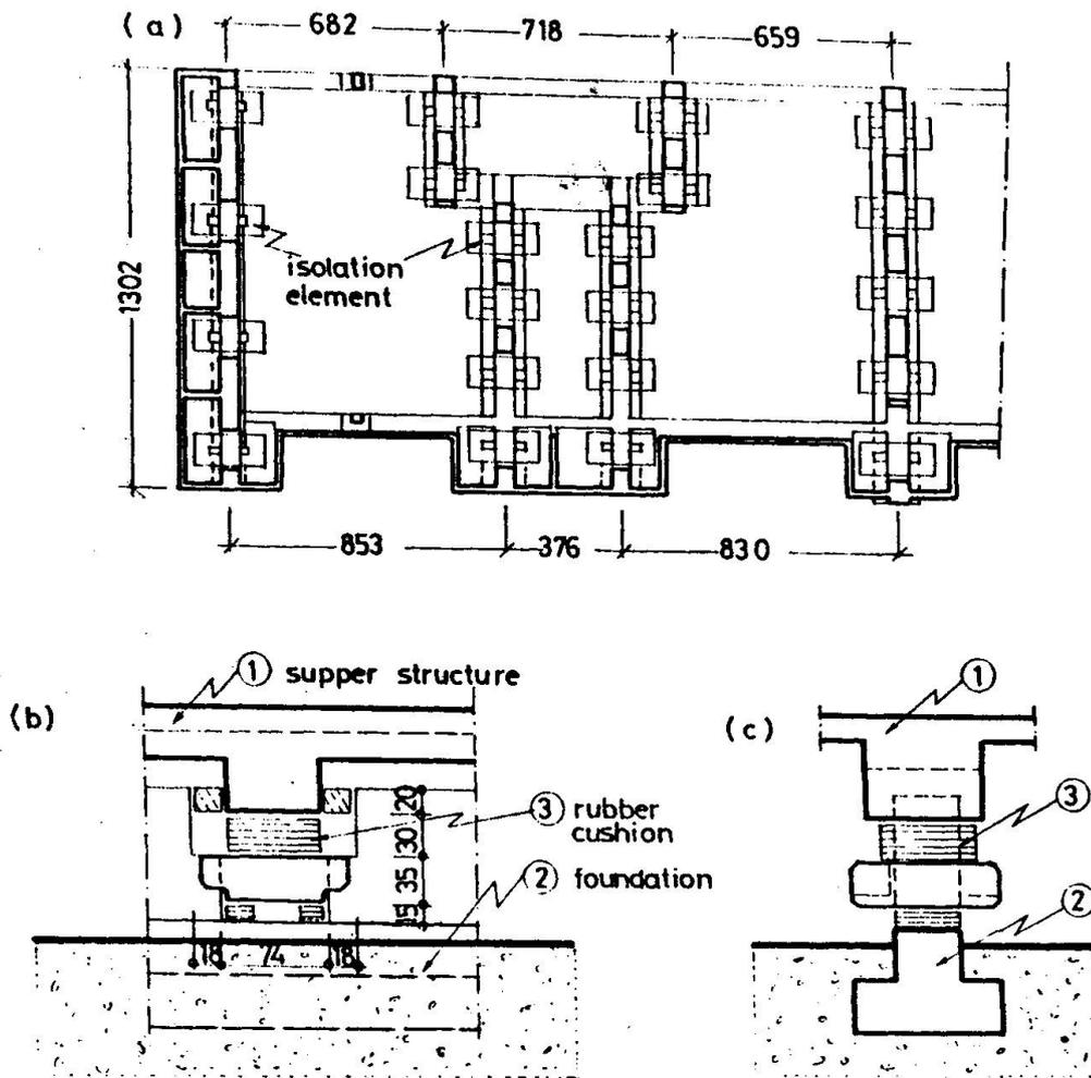
Fig. 3 (a) Partial foundation plan with position of rubber cushions
