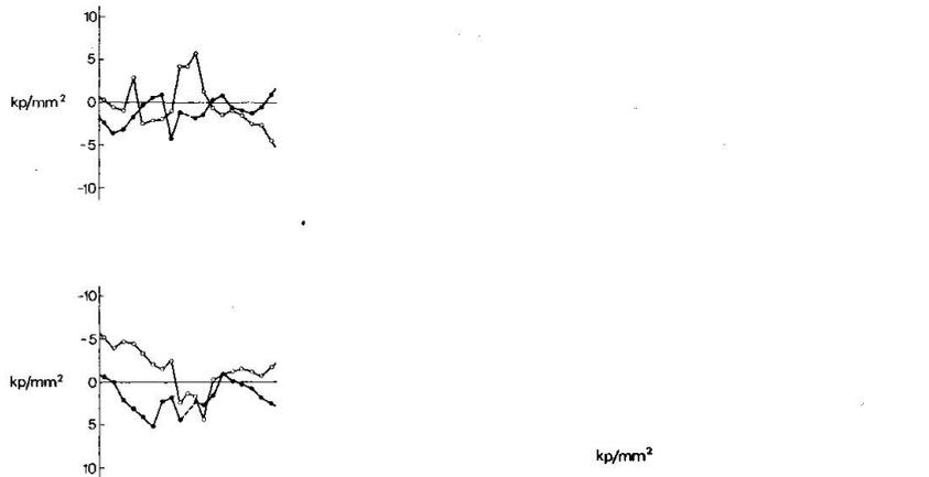
Fig. 7 Residual stresses in an HE 200 A shape rotorized using a modified procedure with larger deflections than in normal production
