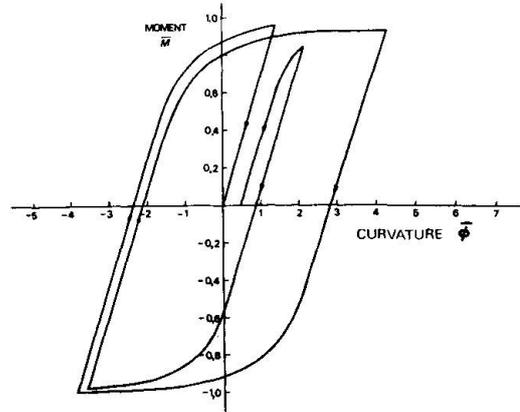
Fig. 15 Typical moment-curvature history as calculated for a simulated rotorizing
