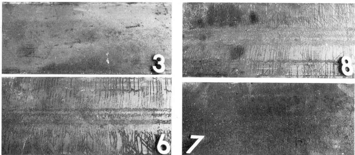
Fig. 2 Mill scale on flange outer surfaces of HE 200 A shapes. As-rolled ("3"), normal rotorizing ("6"), twice rotorizing ("8"), and modified rotorizing ("7").
