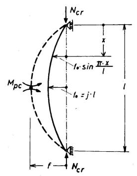
fig. 1: Column with sinusoidal initial out of straightness.
