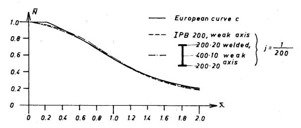
fig. 5 : European buckling curve c compared with approximate theory
