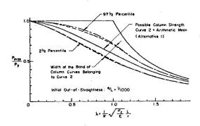
Fig. 6 Possible Column Strength Curve 2, and the Statistical Properties of the Band of Column Curves that Belong to It
