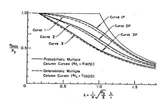
Fig. 11 A Comparison of the Two Sets of Deterministic and Probabilistic Multiple Column Curves
