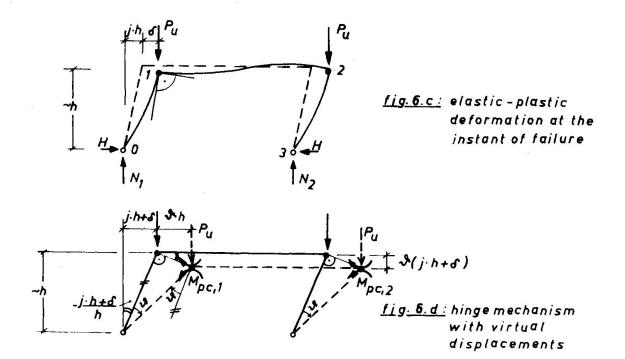
Instead of crooked columns an initial displacement j.h of the column tops is assumed. The frame shall be designed in such a manner that the moment capacity of the columns is less than that of the girder. Therefore the plastic hinges shall performe in the columns.
