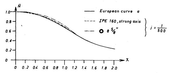
fig. 3. European buckling curve a compared with approximate theory
