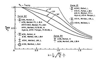
Fig. 10 Possible Maximum Strength Multiple Column Curves,
