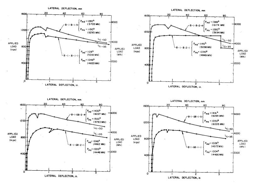
Fig. 9a Pinned-End Column Test Results
