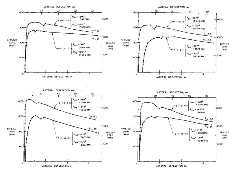
Fig. 9b Pinned-End Column Test Results
