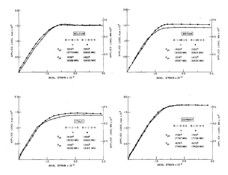
Fig. 7 Stub Column Test Results
