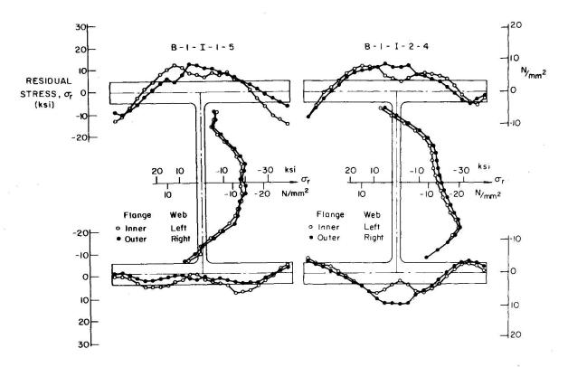
Fig. 5c Residual Stresses in HEM 340 (Italy)
