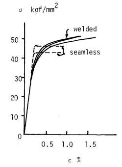
Fig.3  $\sigma - \varepsilon$  curve from stub-column tests
