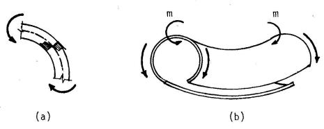
Fig.1 Cold Forming of Steel Tube
