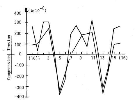
(c) Thermal Residual Stress due to Welding
