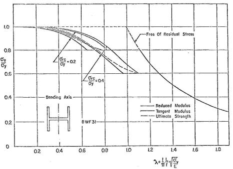
FIG. 12. - COMPARISON OF BUCKLING AND ULTIMATE STRENGTHS
