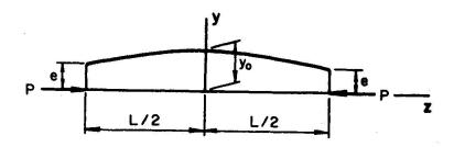
Fig. 1 Eccentrically loaded column
