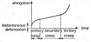
fig. 1: creep behaviour of steel at elevated temp. (schematical)
