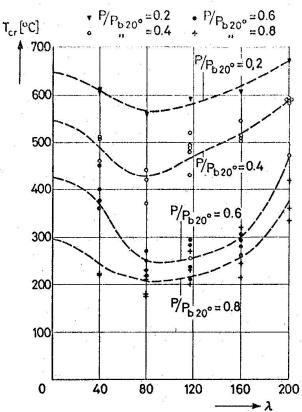
Relation between critical temperature and stend nessratio at different values of  $P_{b\,20}^{\circ}$  (FeE 2-
