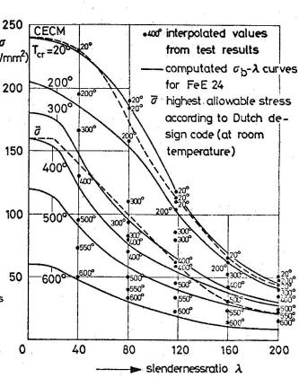
relationship between critical stress and slendernessratio at different temperatures
