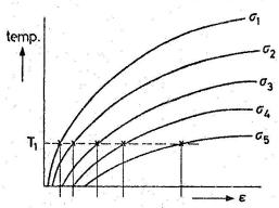
$\varepsilon$ -T diagrams at different stresses  $\sigma_1 < \sigma_5$  (schematic)
