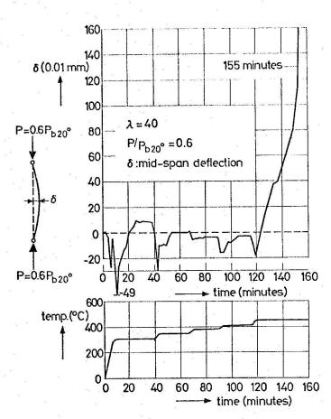
working-method of the creep-buckling-test fig.5
