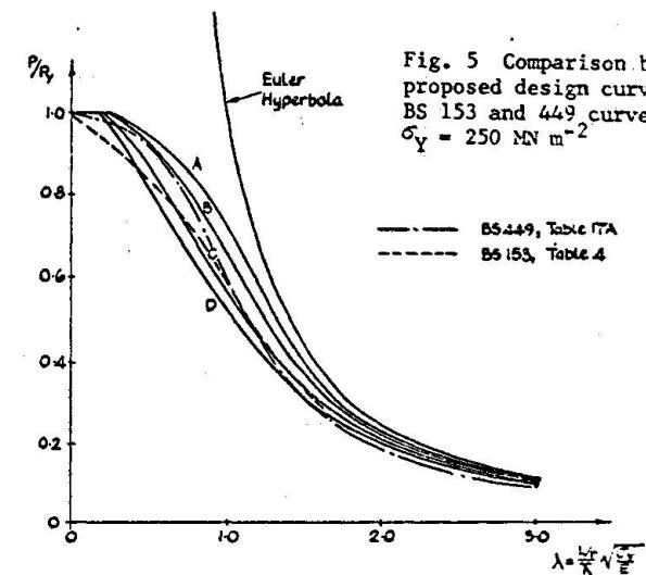
Fig. 5 Comparison between proposed design curves and the BS 153 and 449 curves for  $\sigma_y = 250 \text{ MN m}^{-2}$
