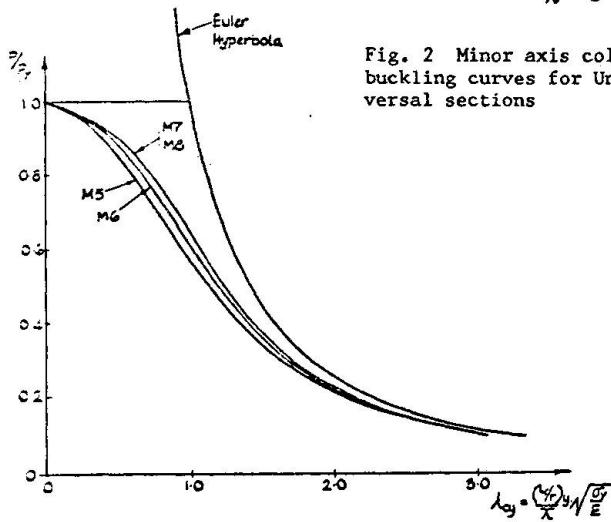
Fig. 2 Minor axis column buckling curves for Universal sections
