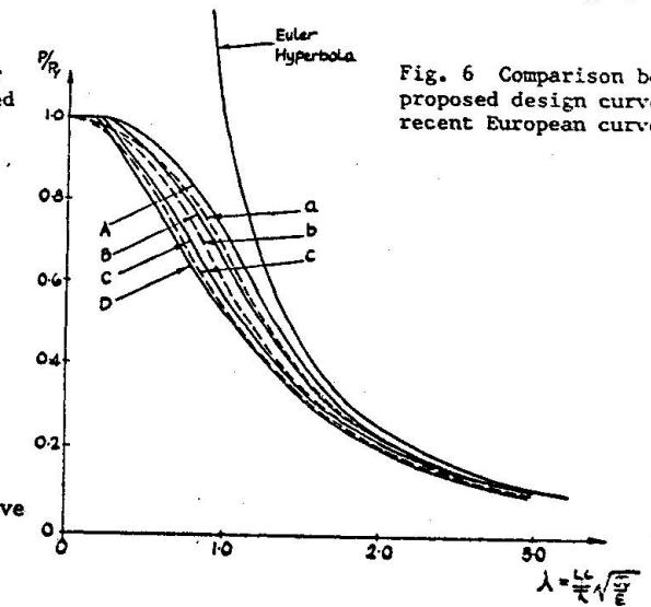
Fig. 6 Comparison between proposed design curves and recent European curves
