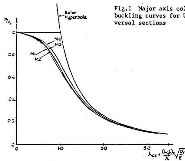
Fig. 1 Major axis column buckling curves for Universal sections
