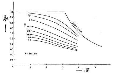
Fig.10 Column Curves of Rectangular Sections
