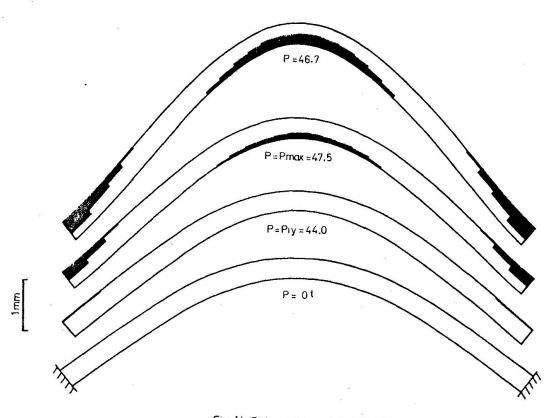
Fig. 14 Deformations of R8026 Specimen
