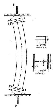
Fig.1 Compression Test Arrangement
