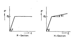
Fig 3 Assumed Stress Strain Diagrams
