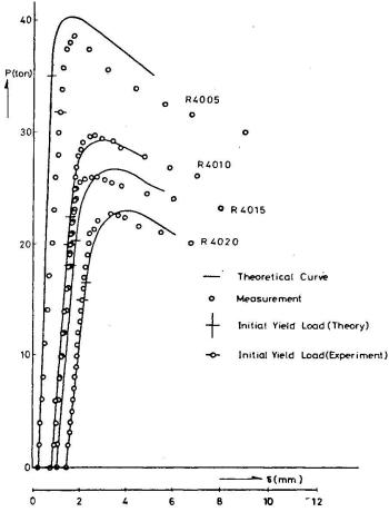
Fig 5 Load-Central Detlection Curves (R40 Series)
