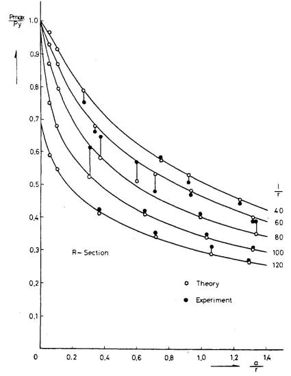
Fig.8 Relation between Maximum Loads and Initial Deflections of Rectangular Sections
