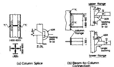
Fig.1 Details of Welded Joints
