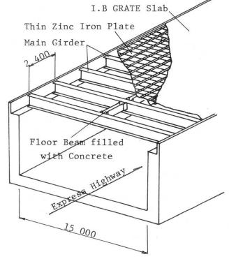
Fig. 13 Schematic View of Box-Culvert
