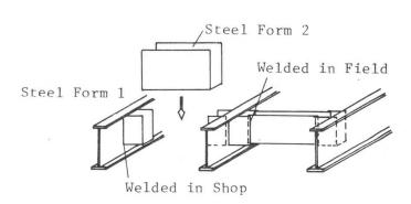
Fig. 4 Erection of Steel Forms
