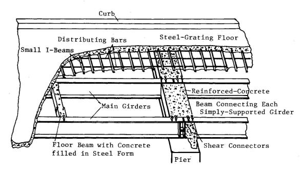
Fig. 1 Schematic View of Composite Girder
