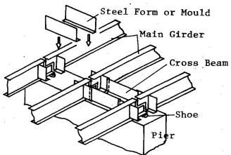
Fig. 7 Details of Connection
