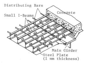
Fig. 3 Details of Grating Floor System
