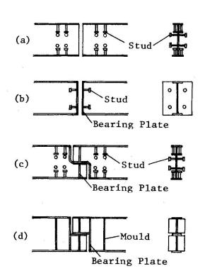
Fig. 9 Details near the Ends of Main Girders
