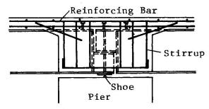
Fig. 8 Placement of Bars
