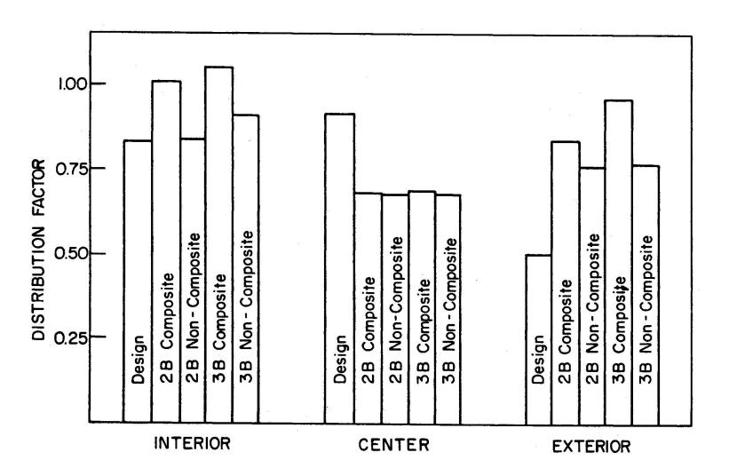
Fig. 2 Distribution Factors, Design vs. Finite Element Analysis
