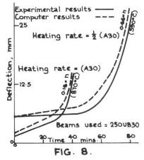
Test results and the associated theoretical prediction are plotted in Figure 8. It can be seen that there is good correlation between theory and experiment in this case. It was found that the applied stress level has a great bearing on the failure temperature and time (Fig. 8) and, as said previously, the fire rating of the component can be greatly changed by changing applied stress levels.
