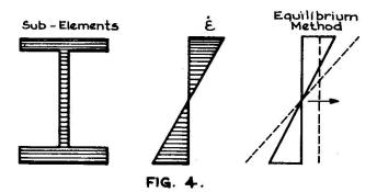
The beam is sectioned as shown in Figure 4 and each section is assumed to be a tension or compression element which has constant stress, strain, strain rate and temperature over its sub-area at any given time. These elements have their behaviour governed by equations (1) and (2). For
