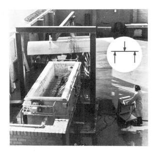
The internal dimensions of the furnace are  $1.2 \text{ m} \times 4.2 \text{ m}$  with reaction supports at 3 m centres. The loading procedure is as shown in the overlay on Figure 15.
