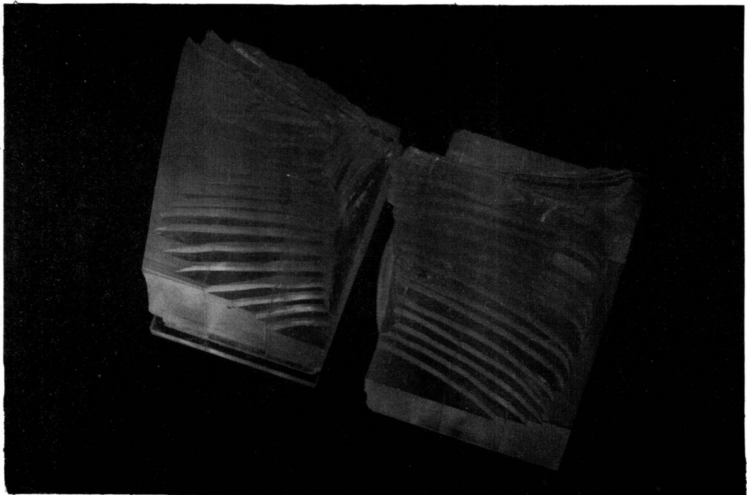
Figure 12 - Negative Mold of Arch Dam and Valley
