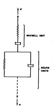
Fig. 3. Viscoelastic model for concrete; pseudo-time t' rather than the time t is used as the time variable.
