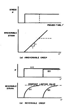
Fig. 2. Reversible and irreversible components of creep plotted against t'.
