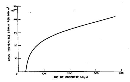
Fig. 7. Basic irreversible creep per unit stress from reference [15].
