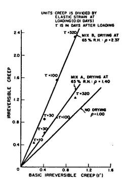
Fig. 4. Irreversible creep at relative humidities of 95% (basic creep) and 65%. Mix A has a water cement ratio of 0.28 while for mix B the ratio is 0.55. The aggregate/cement ratios were 2.0 and 5.5 respectively.
