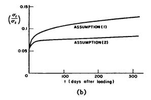
Fig. 9.  $\sigma_{\mathbf{r}}$  for concrete cylindrical core at various values of t' and t, for two assumptions regarding Poisson's ratio.
