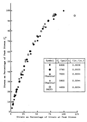
Fig. 3 - Compressive Stress-Strain Curves for Microconcretes
