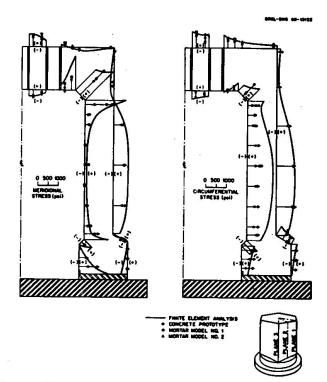
Fig. 12 - Comparison of meridional and circumferential surface stresses in plane 2 for prototype and models subjected to internal pressure of 500 psi. Predictions based on two-dimensional analysis.
