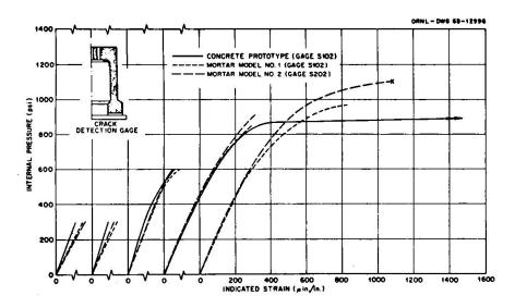
Fig. 17 - Comparison of indicated behavior for meridional crack- detecting strip across haunch of concrete prototype and microcomcrete model.
