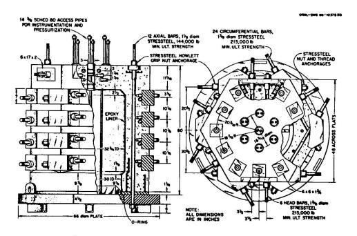
Fig. 8 - Design Details of Concrete Prototype Vessel
