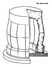
Fig. 13 - Cracking and deformation patterns
