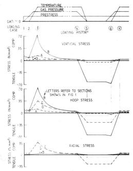
FIG 2 OLDBURY VESSEL APPROXIMATE STRESS HISTORIES AT THE LINER FACE OF VESSEL SECTIONS A-A,B-B,C-C, AND D-D SHOWN IN FIG 1
