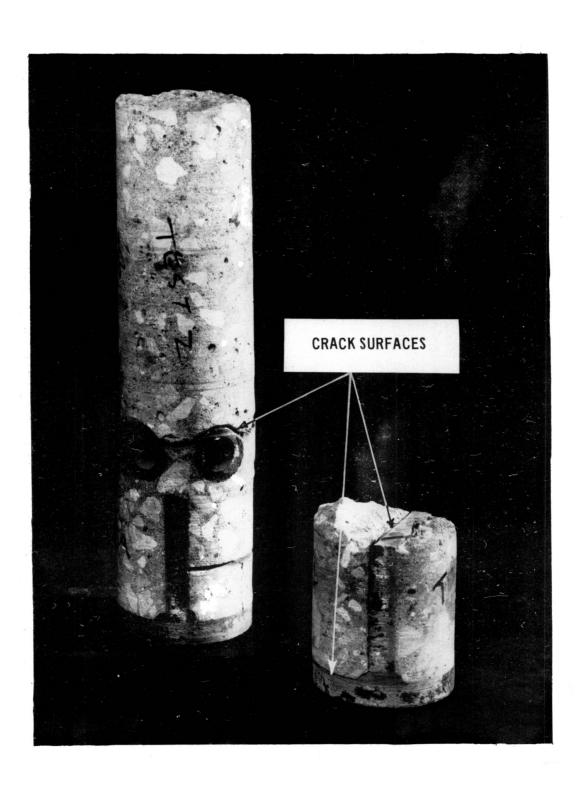
FIG. 14 CORES 1/3 (RIGHT) AND 2/5 SHOWING CRACK SURFACES
