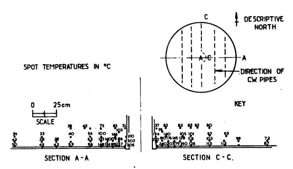
FIG. 10 TEST 3 TEMPERATURES IN THE MODEL AVERAGED FROM VALUES AT DAYS 21, 22, 24, AND 28.
