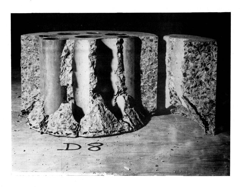
FIG. 10 1/10th Scale Model Boiler Closure Showing Failure Planes
