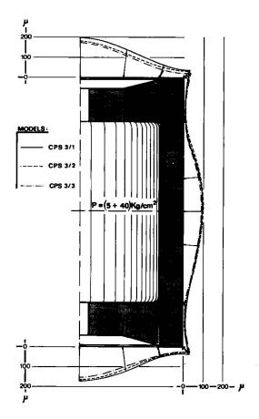
FIG. 8 COMPARISON BETWEEN THE OUTSIDE SURFACE DEFLECTIONS FOR AN INTERNAL PRESSURE
