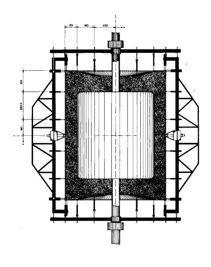
WTK 5 HOTTINGER TYPE DISPLACEMENT TRANSDUCER
