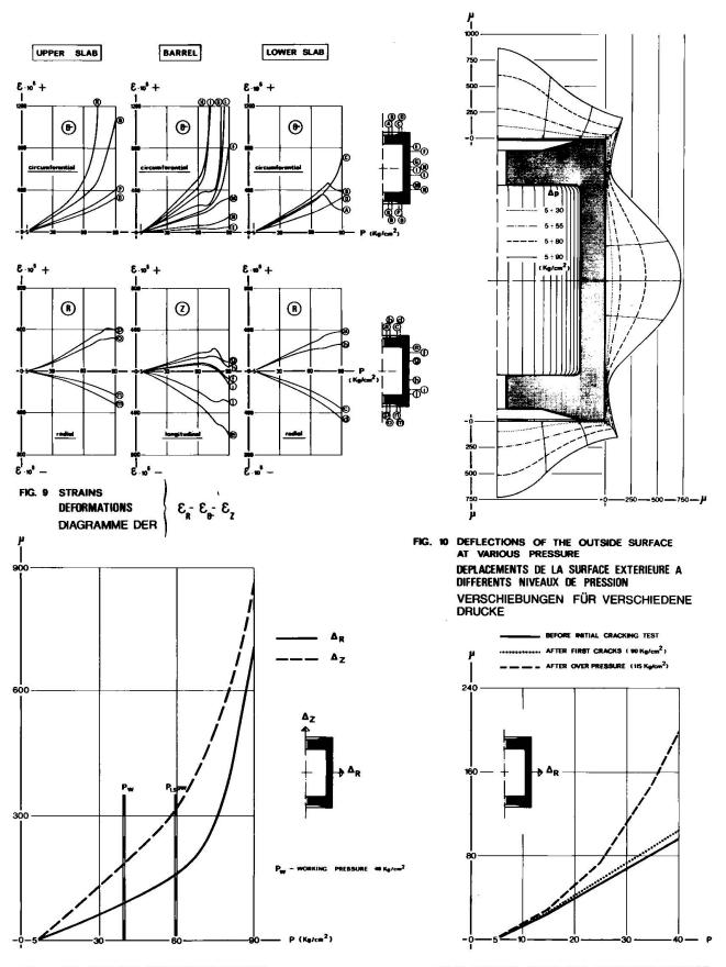
FIG. 11 TOP SLAB AND AEQUATOR DEFLECTIONS
