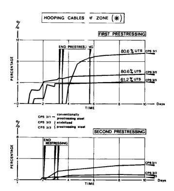
FIG. 6 LOAD LOSSES AT CABLE ANCHOR HEADS
