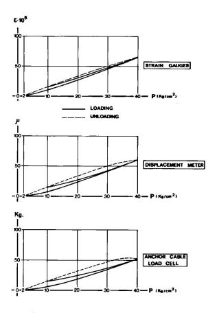
FIG. 7 TYPICAL BEHAVIOUR OF THE MODEL DURING LOADING CYCLES
