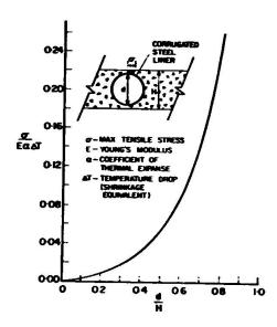
Figure 19 - Effect of Shrinkage Around Circular Voids
