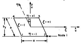
Figure 6 - Special Parallelogram Finite Element
