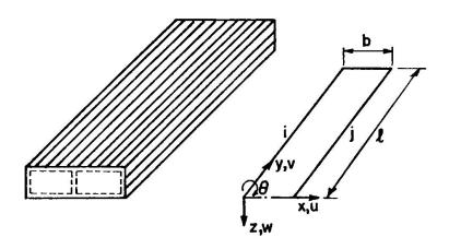
Figure 2 - Typical Finite Strips for Box Girder
