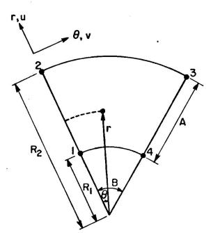
Figure 9 - Special Annular Element
