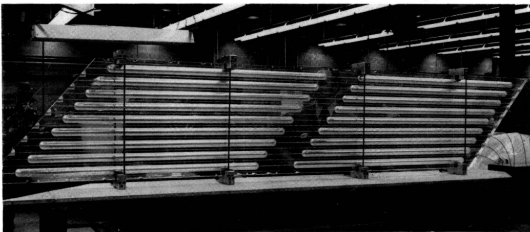
Figure 21 - Two Span Plexiglass Model of a Post-Tensioned Voided Skew Bridge Slab (1/24)
