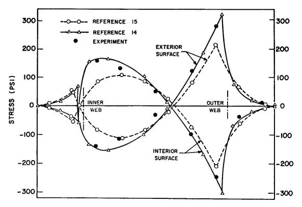
Figure 11 - Radial Stresses in Top Flange
