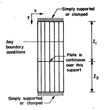
Figure 5 - Longitudinal Strips for Continuous Span Analysis
