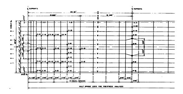
Figure 22 - One Half Plan View of 1/36 Scale Model Showing Gauge and Cable Locations
