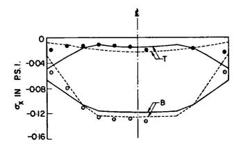
Figure 25 - Longitudinal Stresses Along Transverse Grid Line 4
