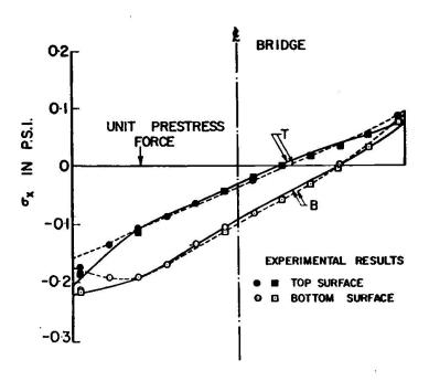
Figure 23 - Longitudinal Stresses Along Transverse Grid Line 4 Unit Prestress in Cable 1
