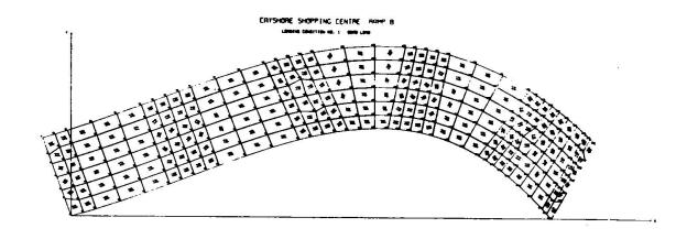
Figure 16 - Principal Stress Plot for a Curved Voided Bridge using WATSA-4
