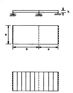
Figure 3 - Transverse Strips for Continuous Span Analysis
