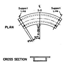
Figure 10 - Geometry of Box Girder Model
