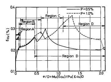
Fig. 7 e- $\epsilon_{CU}$  relations for rectangular column section of p=0.5% and 1% (Curve I concrete stress-strain relation and  $F_y$  = 4000 kg/cm<sup>2</sup> are used in calculation)
