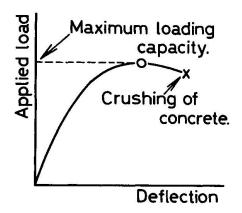
Fig. 1 Load-deflection curve of reinforced concrete member
