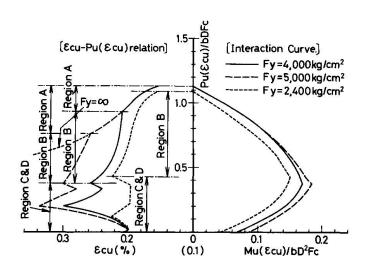
Fig. 9 Effects of the yield strength of reinforcement upon  $\epsilon_{\text{CU}}$  -  $P_{\text{U}}(\epsilon_{\text{CU}})$  - $M_{\text{U}}(\epsilon_{\text{CU}})$  relations of rectangular column section of p = 0.5% (Curve I concrete stress-strain relation is used in the calculation)
