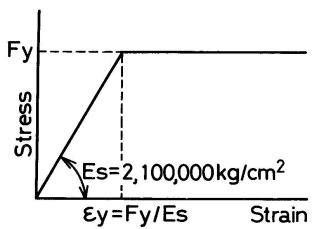
Fig. 4 Stress-strain curve of reinforcement
