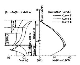
Fig. 8 Effects of the type of concrete stress-strain curve upon the compressive fiber strain,  $\varepsilon_{\text{CU}}$ , at ultimate strength (p = 0.5%,  $F_{\text{V}}$  = 4000 kg/cm<sup>2</sup>)
