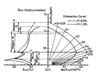
Fig. 6  $\varepsilon_{cu}$  -  $P_u(\varepsilon_{cu})$  -  $M_u(\varepsilon_{cu})$  relations for rectangular column section (Curve I concrete stress-strain relation and  $F_V = 4000 \text{ kg/cm}^2 \text{ are used in}$ cálculation)
